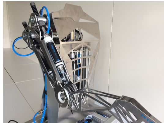
Fig. 1. Real robot model of a human arm consisting of two joints (shoulder and elbow), which are articulated by five pneumatic muscle-spring units (MSUs), allowing movements within the sagittal plane (2D). The two joints are driven separately by two monoarticular MSUs each. Additionally, a fifth MSU acts as a biarticular muscle over both joints, performing shoulder anteversion and elbow flexion.
