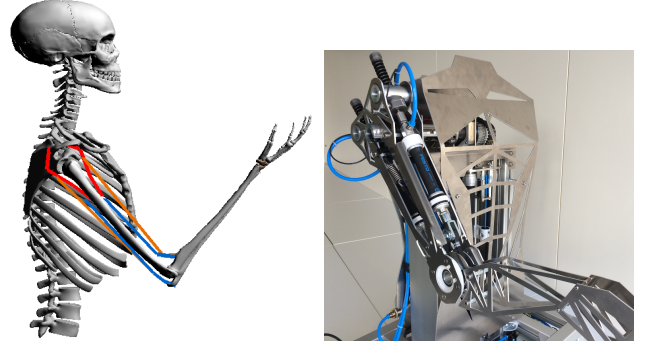
Fig. 2. Left: Simulation model of human arm with elbow and shoulder joint. Red lines are the two monoarticular shoulder muscle tendon units (MTUs), orange the two biarticular ones and blue depicts the two monoarticular elbow MTUs. Right: Real muscle-driven robot with two joints, articulated by five pneumatic muscle spring units (MSUs).
