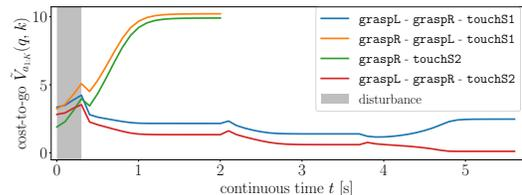
Fig. 3. Predicted cost-to-go  $\tilde{V}_{cost}(q, k)$  of (initially) feasible action sequences over continuous time  $t$ , based on which the controller chooses a discrete action sequence to execute; transitions to next actions are at  $t = 2$ s and  $t = 3.7$ s.
